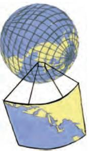
A nautical chart is flat, but it represents a round surface. Geodesy is the science of defining the earth's shape, which is a slightly squashed globe called an ellipse.
